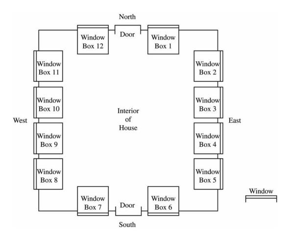
In the interior of the house, each window is surrounded by a window box to capture and measure the amount of heat coming in through that window and to isolate the heat gain for each window.
